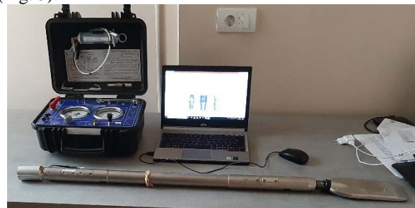
Figure 3. Seismic dilatometer equipped with additional sensors for P-wave measurements (SPDMT)
