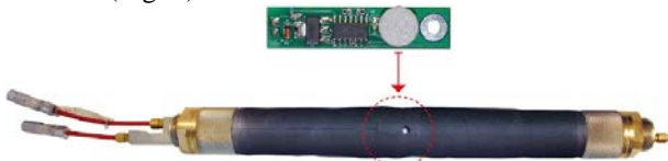
Figure 4. Electronic card with integrated sensor for pore pressure measurement and its place on the sheath (SA Jean Lutz®)
