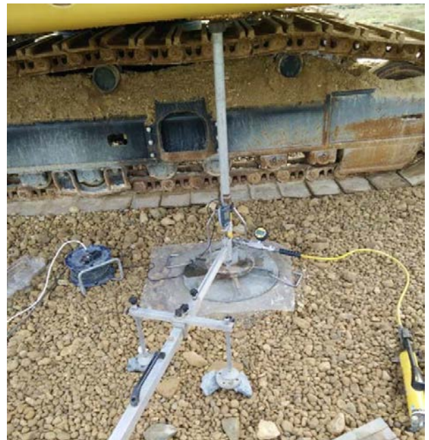
Figure 7. 600mm PLT test on a gravel bed.
