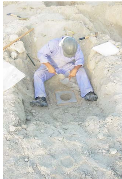
Figure 6. Execution of a sand replacement test.
