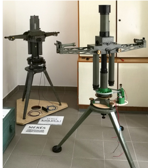
Figure 2. Two types of historical torsion balances for field measurements, the Auterbal on the left side, and the Eötvös-Pekár torsion balance on the right side can be seen.
