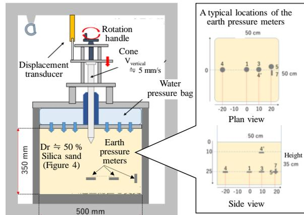
Figure 10. Outlines of a preliminary calibration chamber test.
