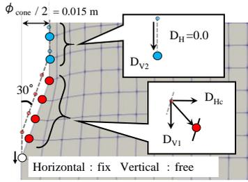
Figure 3. Calculated procedures of cone penetration.
