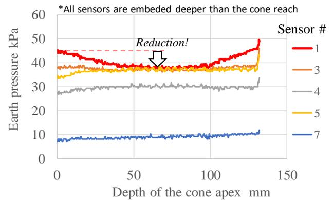
Figure 11. A typical measurement result of earth pressures.
