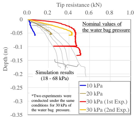
**Figure 12.** Comparisons of all the results obtained from both experiment and numerical simulations conducted at different over burden pressures.
