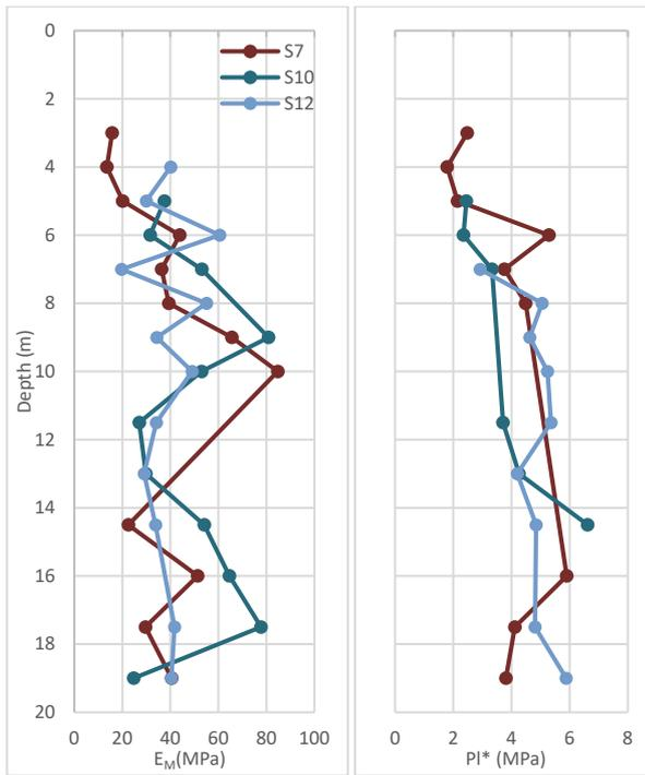
**Figure 7.** Menard moduli ( $E_M$ ) and limit pressures ( $p_{LM}^*$ ) inferred from the pressuremeter tests performed using the TUBA® system. Only the measurements that are used in the statistical analysis are represented.
