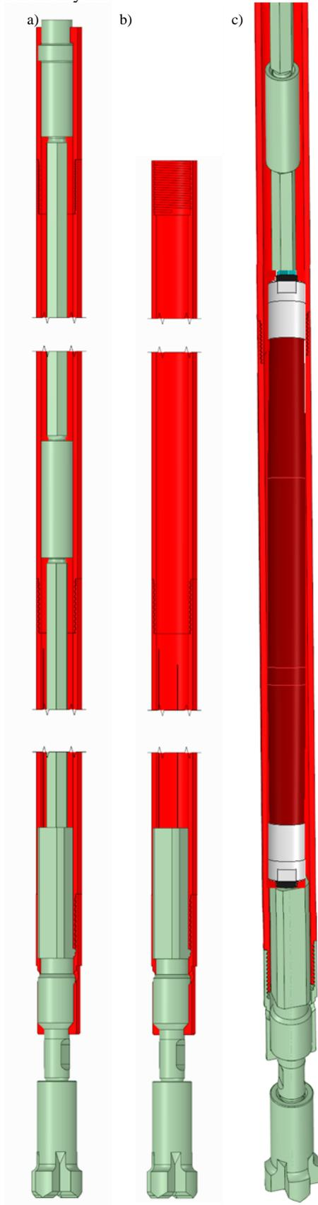
**Figure 1.** TUBA® system. a) The borehole is carried out and the casing is advanced while drilling. The lowest casing is slotted. b) At the end of the drilling, the drill rods are removed. c) The pressuremeter probe is moved down in the slotted tube and the pressuremeter test is performed. At the end of each test, the whole system is raised up to the next test location.
