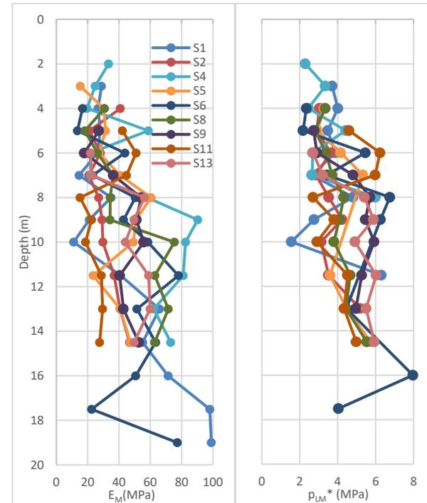
**Figure 6.** Menard moduli ( $E_M$ ) and net limit pressures ( $p_{LM}^*$ ) inferred from the pressuremeter tests performed using the Driven Slotted Tube procedure (RPM). Only the measurements that are used in the statistical analysis are represented.
