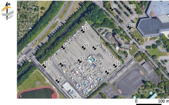
**Figure 4.** Map layout of the boreholes where pressuremeter tests were carried out.
