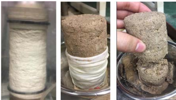
Figure 14. Shape of S2 specimen after CD test (confining pressure:200kPa, sheared up to axial strain of 20%)
