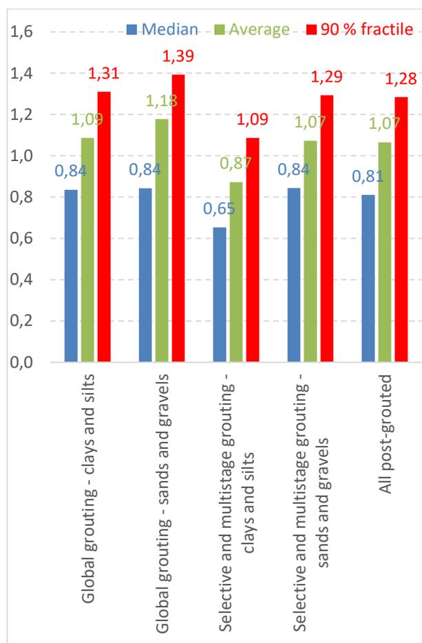
Figure 8. Average, median and 90 % fractile for clays and silts then sands and gravels
