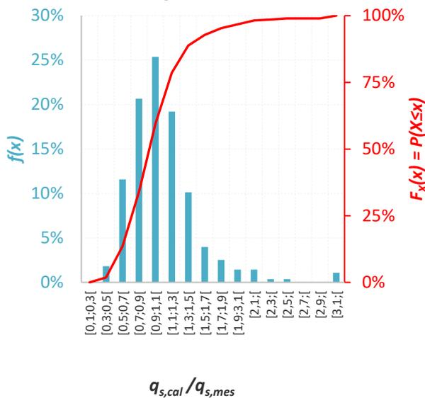
Figure 6. Histogram and distribution functions of unit shaft friction ratio
