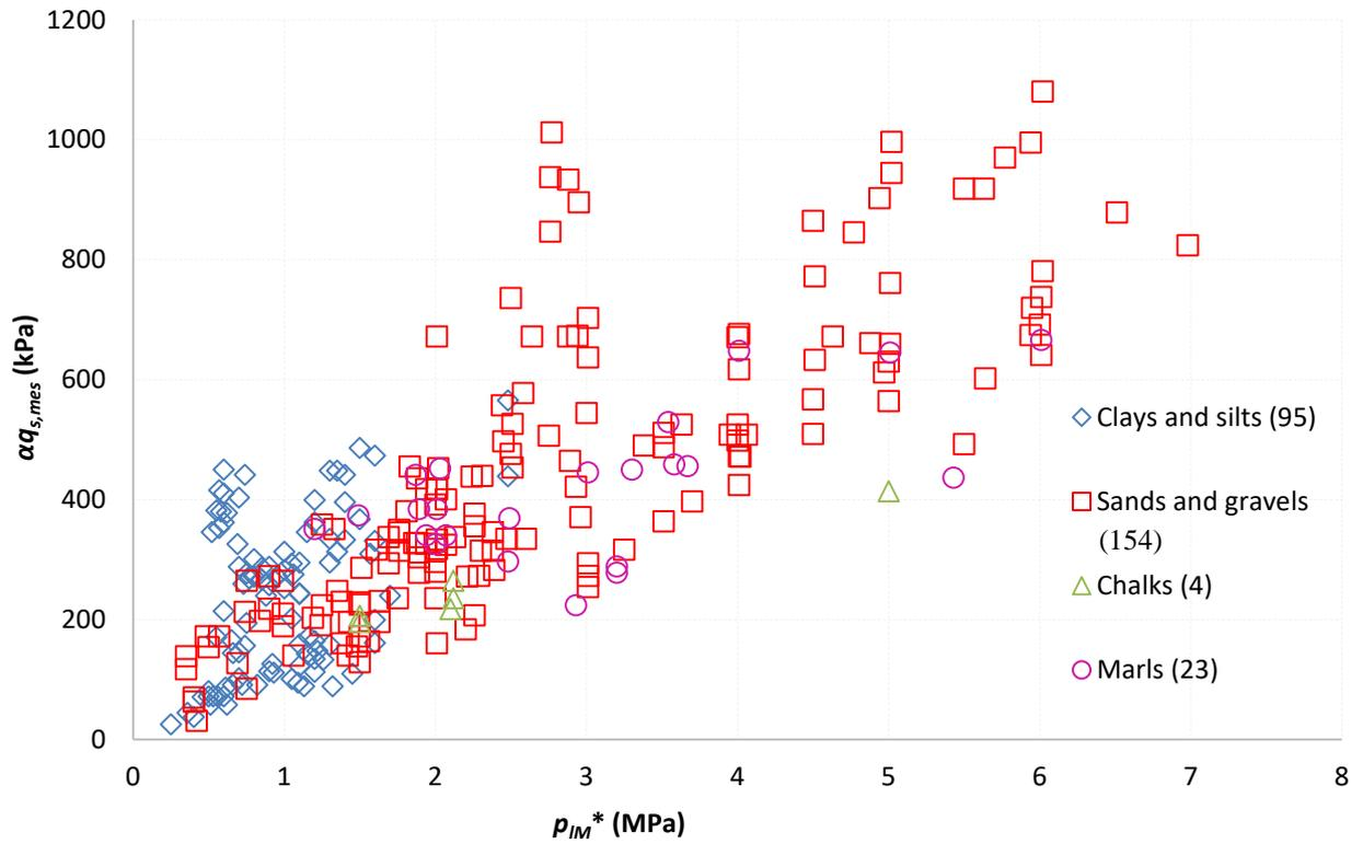
Figure 2. Obtained results (by ground types – 276  $q_s$  measurements)
