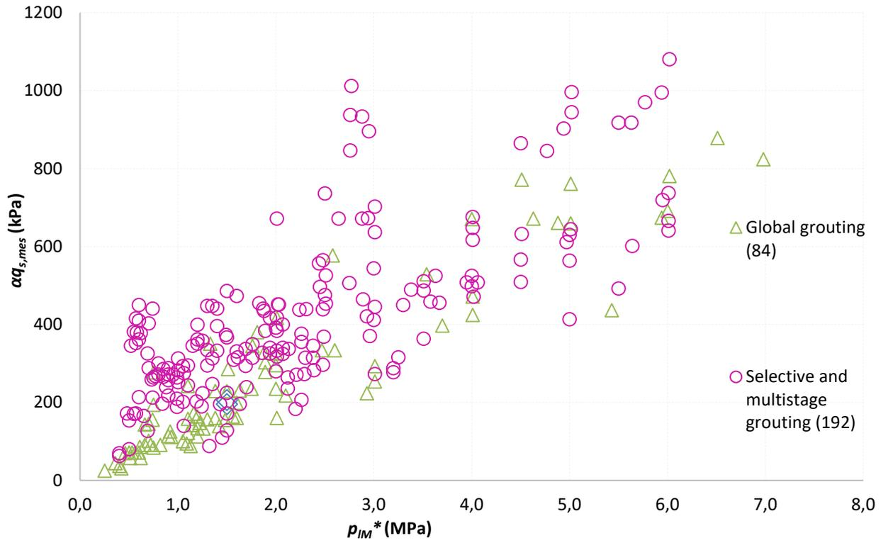
Figure 3. Obtained results (by execution conditions – 276  $q_s$  measurements)
