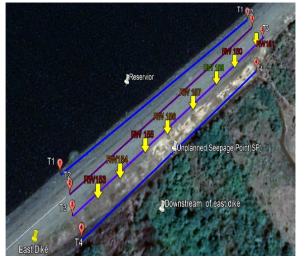
Figure 3: Four traverse lines for resistivity measurements
