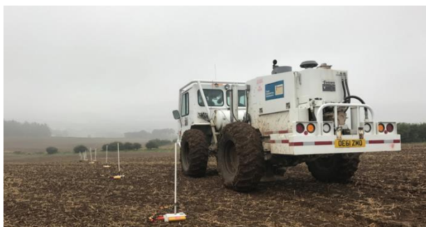
Figure 4: Wireless seismic receivers capture the transmitted signal from a vibroseis seismic source reflected from the subsurface to yield seismic reflection imagery. The combination of these technologies provided a low environmental impact approach for the tunnel investigation and minimal disruption to local communities. An equivalent investigation based on a traditional explosives approach could have involved about 17000 shot holes and up to 10 t of explosives.
