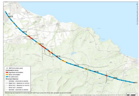
Figure 8: Linear risk map of deformed strata based on 2017/2018 Fugro seismic campaign. Zoning of the tunnel route focussed risk mitigation decisions on those parts of the route with significant deformation within the tunneling interval.
