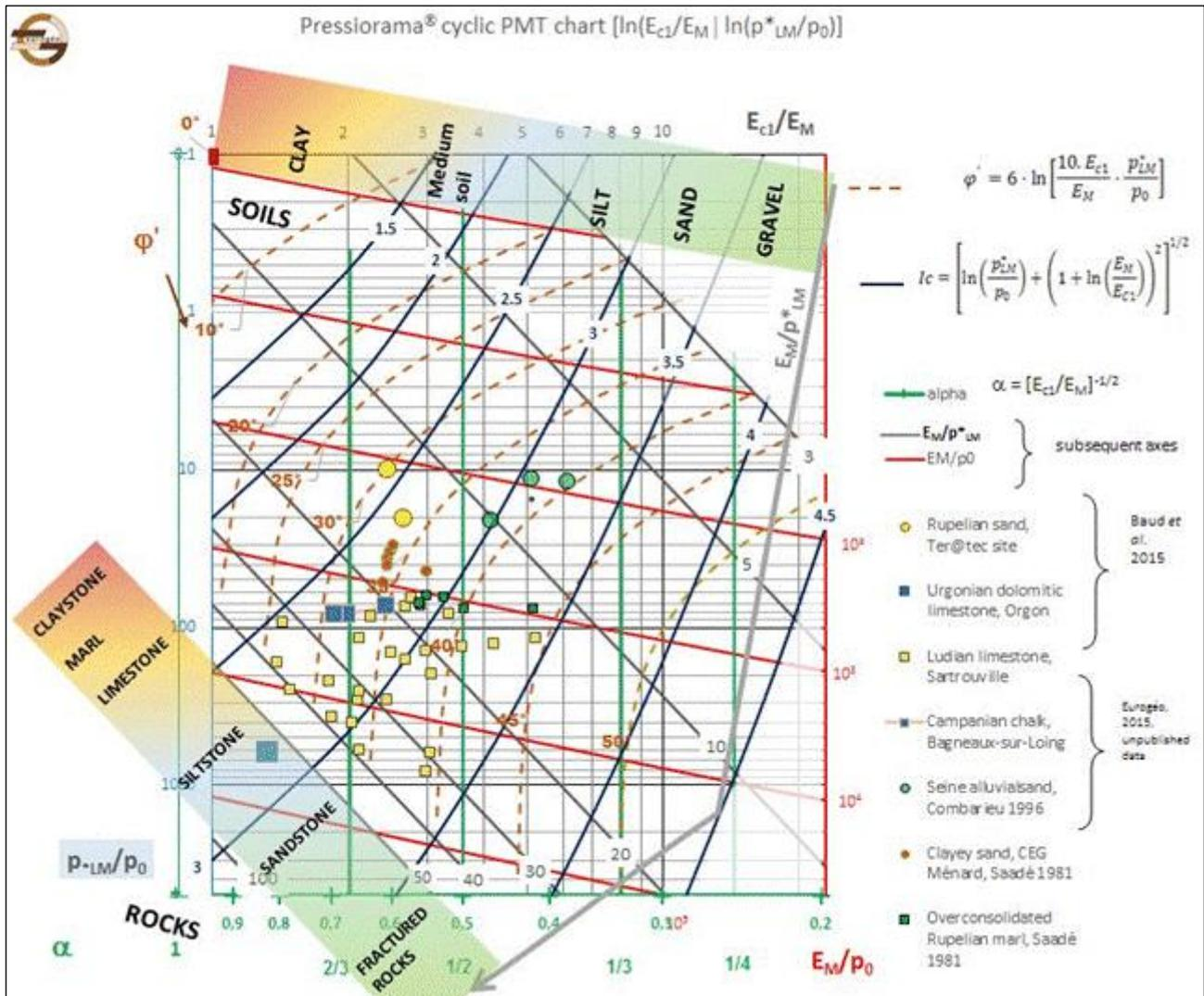
Figure 7. Soils and rocks classification from cyclic PMT
