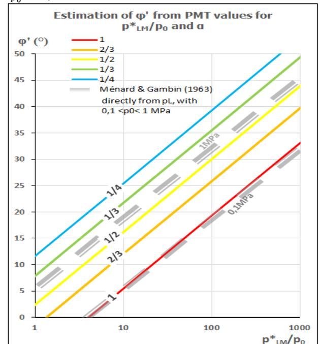
Figure 4. Estimation of  $\phi'$  from Pressuremeter test.
