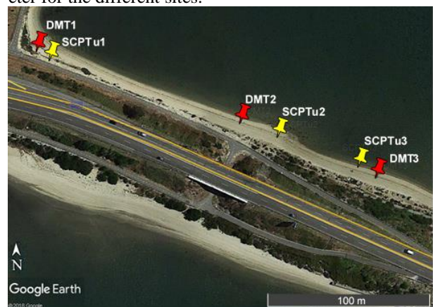
Figure 1. Map of the experimental site and location of the SCPTu and DMT tests
