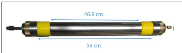
Figure 2. Monocell probe with vulcolan rings
