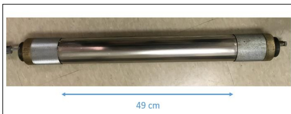
Figure 3. Monocell probe with metallic rings
