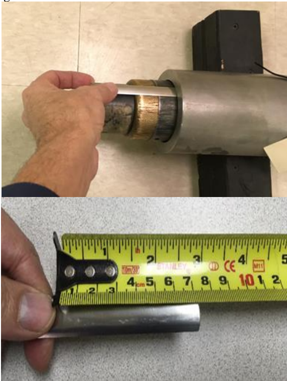
Figure 5. Measuring CL with a steel strip
