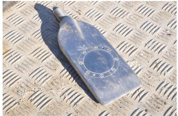
Figure 8. DMT Blade used in fine grained soils with some gravel showing some scratching that may damage the membrane.
