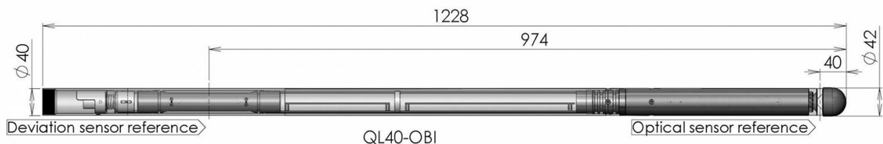
Figure 1. Optical scope OBI40-2G.
