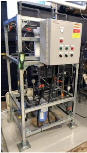
Figure 6. Liquid-Cel de-airing system
