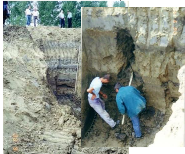
Figure 7. Opening of the sand boil
