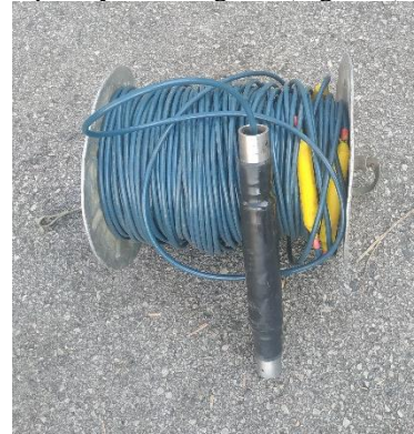
Figure 1. Geo-Log Ltd developed downhole unit without pneumatic system
