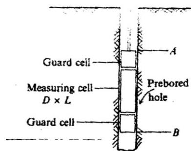
Figure 1. PMT device
