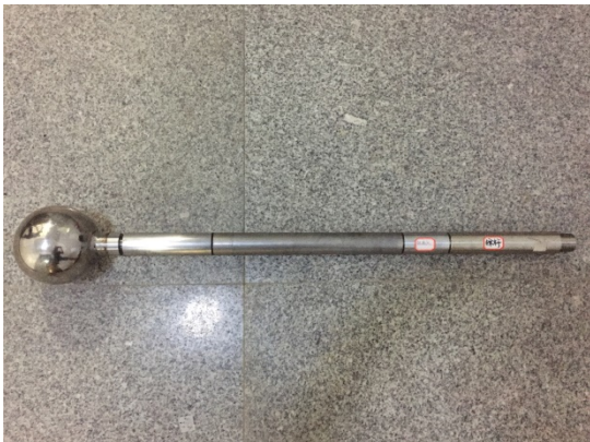
Figure 2. Ball full-flow penetrometer developed by Southeast University
