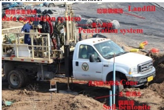
Figure 1 CPTU field test diagram of soil-bentonite wall
