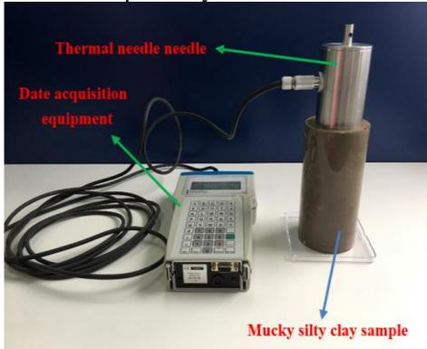
**Fig. 1** Mucky silty clay specimen and thermal needle system
