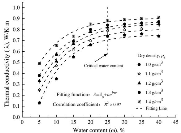
**Fig. 2** The relationship between thermal conductivity of mucky silty clay and water content
