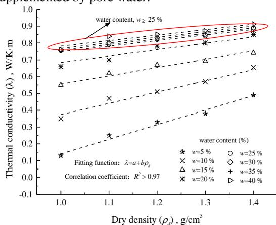
Fig. 3 The relationship between thermal conductivity of mucky silty clay and dry density
