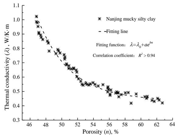
Fig. 4 The relationship between thermal conductivity of mucky silty clay and porosity
