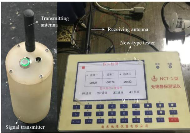
Figure 7. Ground signal transmitter and new-type tester
