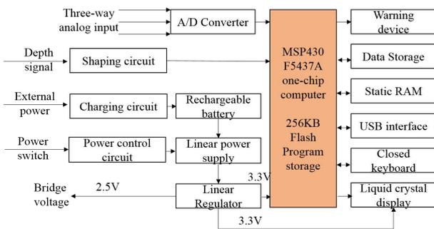
Figure 8. Circuit schematic diagram of the new-type tester
