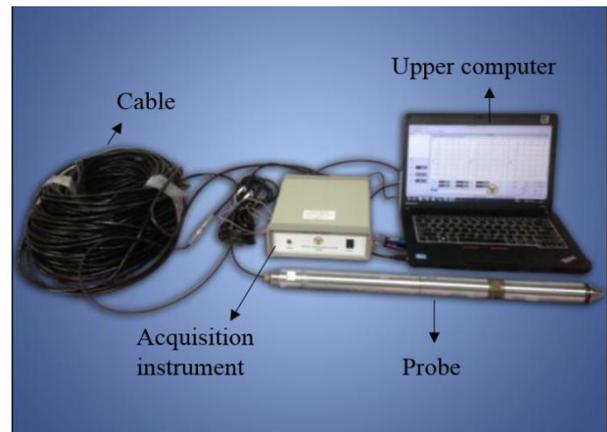
Figure 4. Traditional CPT system with cable
