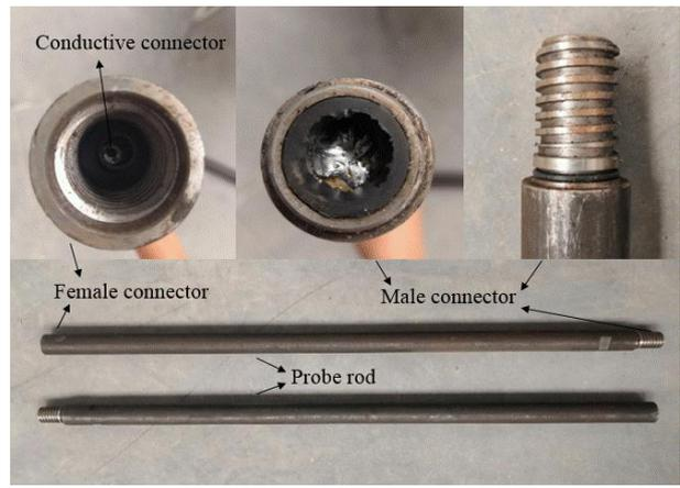
Figure 6. Structural Composition of special probe rod
