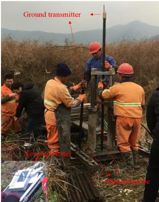
Figure 10. Field Tests of Wireless Static Penetration System
