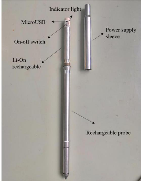
Figure 5. Rechargeable probe for Wireless CPT System
