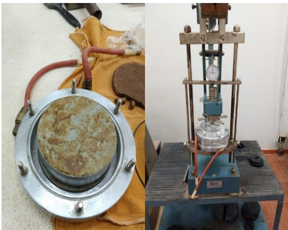
Figure 7. Determination of swelling properties by Constant volume oedometer test procedure.
