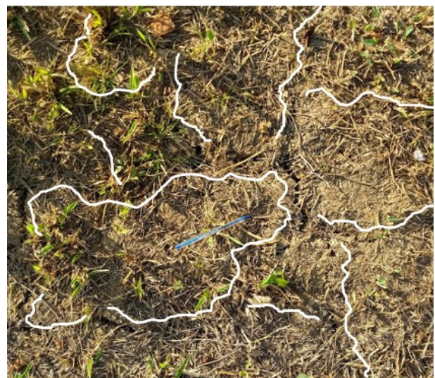
Figure 5. Occurrence of cracking in roughly polygonal patterns at the studied site.
