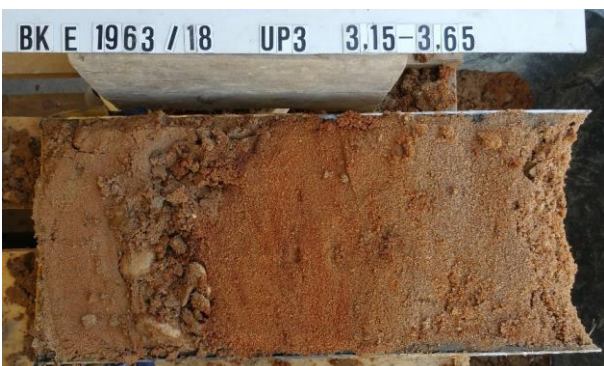
Figure 7. Example of samples of non-cohesive soils taken by the Stoeelben sampler in the unsaturated zone showing the in situ sedimentary structures
