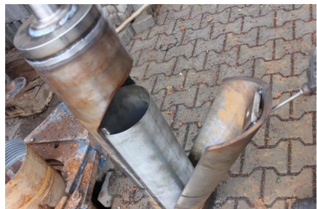
Figure 1. Stoelben sampler made from stainless-steel with liner and window for extraction
