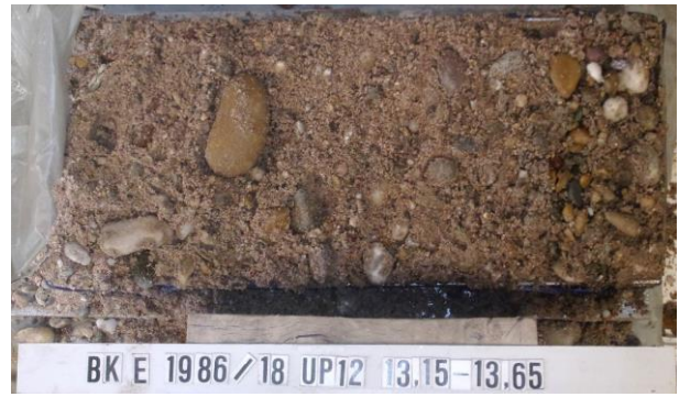
Figure 8. Example of samples of non-cohesive soils taken by the Stoeelben sampler in groundwater
