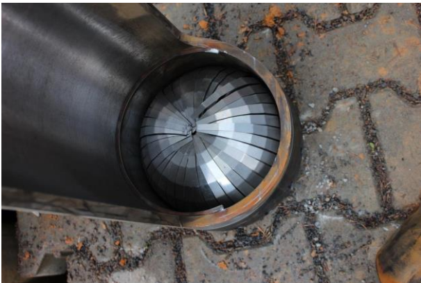
Figure 2. Core catcher at the bottom of the Stoelben sampler
