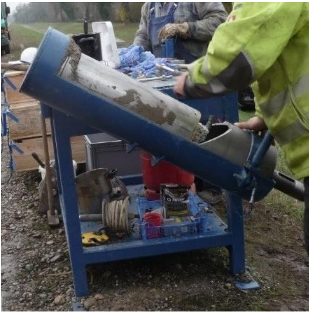
Figure 5. Stoeelben sampler in a special holding device to facilitate the handling and liner extraction
