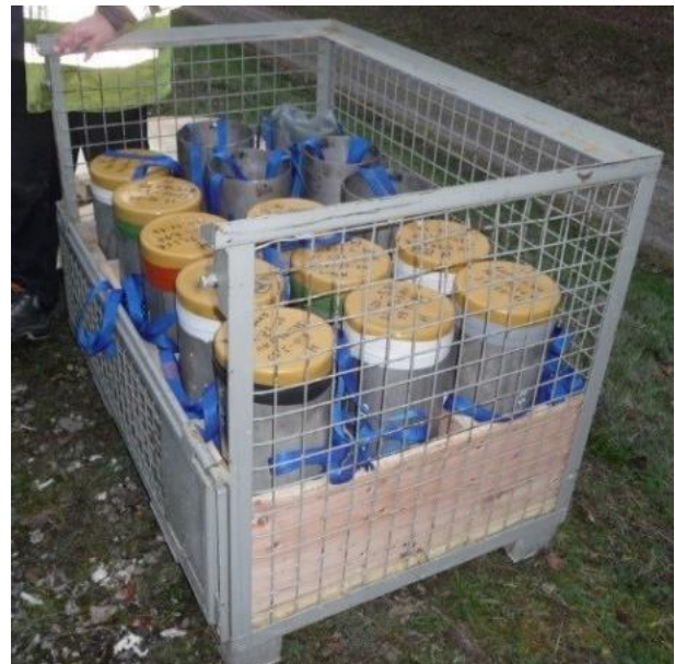
Figure 9. Transport of liner samples according to sampling category A of ISO 22475-1 [1]
