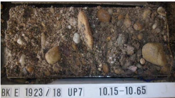
Figure 6. Example of samples of non-cohesive soils taken by the Stoeelben sampler in groundwater
