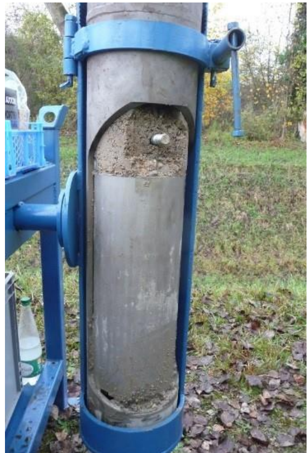
Figure 4. Stoelben sampler with opened window to extract the stainless-steel liner
