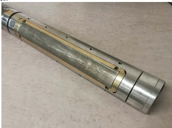
Figure 1. The probe showing one of its two rigid punches diametrically opposed.
